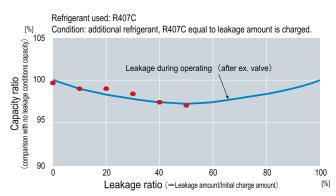
L Safety evaluation for changed refrigerant composition under the worst conditions of cooling machine operation
