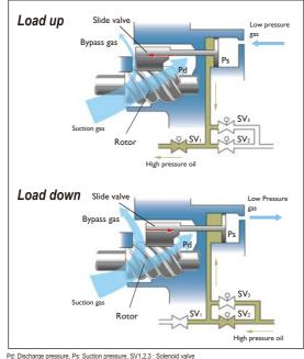
Pd: Discharge pressure, Ps: Suction pressure, SV1,2,3: Solenoid valve
