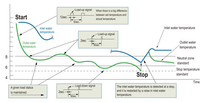
By continuous capacity control by a microcomputer, the air-conditioning load can be finely adjusted as shown in the drawing below and extra energy can be eliminated to ensure energy-efficient operation
